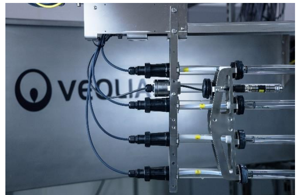
Figure 4: Close-up of UV sensor including optional wiping system
